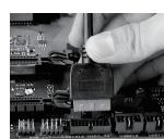
Insert USB3.0 connector to motherboard position
