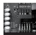
Insert HD Audio connector to motherboard position
