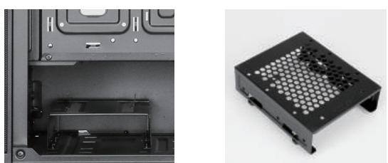
Put SSD on the top of bracket and fix screws from bottom of the bracket
